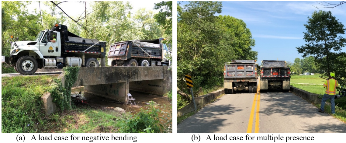
Fig. 3. Typical load cases utilizing both test trucks.
