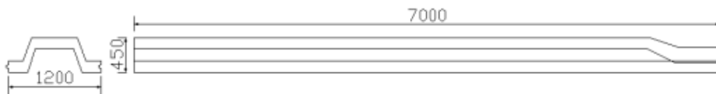
Figure 1. Dimension details of Precast Concrete Sheetpile ST-Series.
