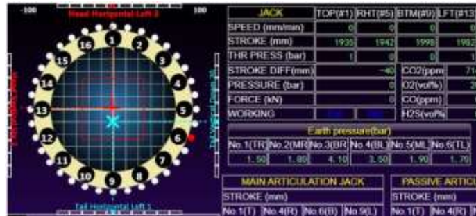
Figure 5. Thrust jack extension details after completion of mining (Enzan display).
