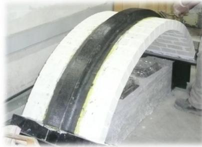
Figure 2. Strengthened arch by  $\Omega$ -Wrap system.
