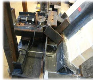
Figure 2. Sliding abutment.
