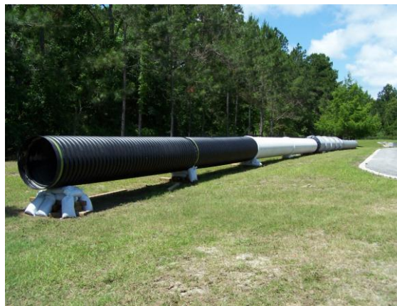
Figure 1. Field Course Comprised of HDPE, PVC, RCP, and CMP.
