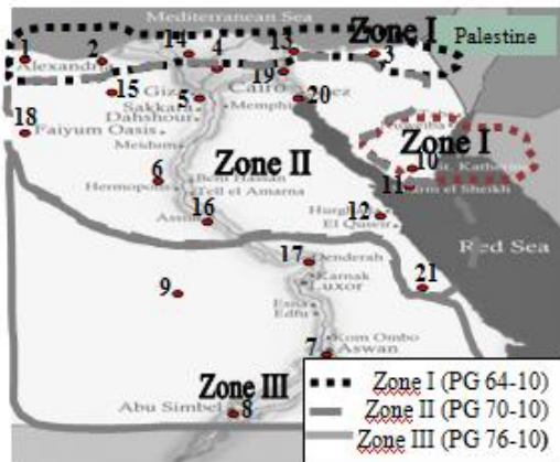
Figure 2. Final performance grades (PG) for high reliability projects all over Egypt (using the LTPP model with a 98% reliability level).
