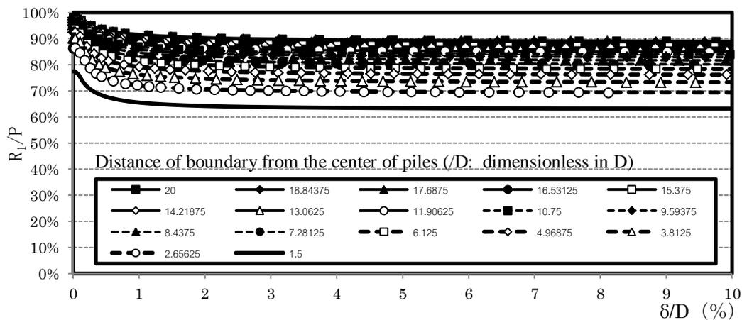
Figure 4. The relationship between the lateral-loading share ratio of the piles ( $R_1 / P$ ) and the relative deformation of the ground ( $\delta/D$ ).
