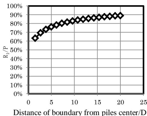
Figure 5. The relationship between the lateral-loading share ratio and the distance from the center of piles in case (A)-② ( $\delta/D=10\%$ ).
