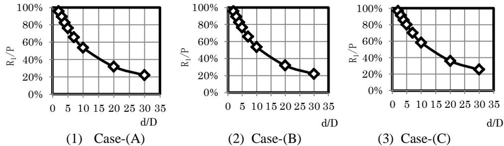
Figure 7. The relationship between pile spacing and lateral-loading share ratio ( $\delta / D=10\%$ ).
