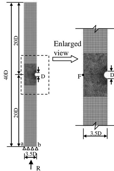
Figure 3. Element meshing ( $d = 7D$ ).
