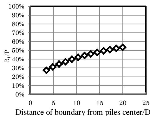
Figure 6. The relationship between the lateral loading share ratio and the distance from the center of piles in case (A)-⑥ ( $\delta/D=10\%$ ).
