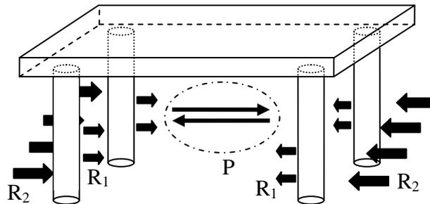
Figure 1. Schematic diagram of liquefaction countermeasure.
