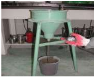
Figure 2. Test of fluidity for grout.
