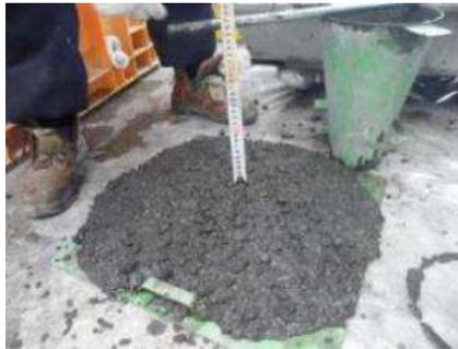
Figure 1. Slump test.
