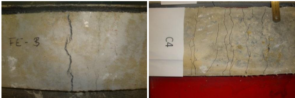
Figure 3. Pictures of cracking in tested EF, and CF panels.
