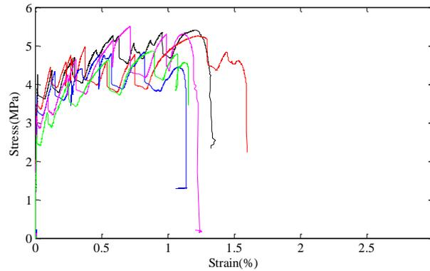
Figure 6. Tensile stress-strain curves of the PVA-ECC at the age of 14 days.
