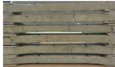
Figure 4. Failure in dog-bone tensile specimens.
