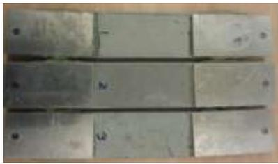
Figure 1. Rectangular-coupon tensile specimen.
