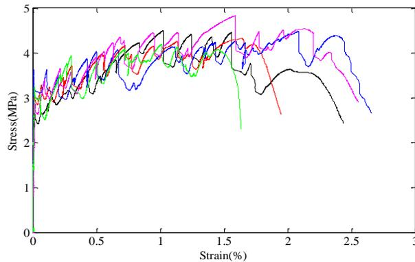
Figure 5. Tensile stress-strain curves of the PVA-ECC at the age of 7 days.
