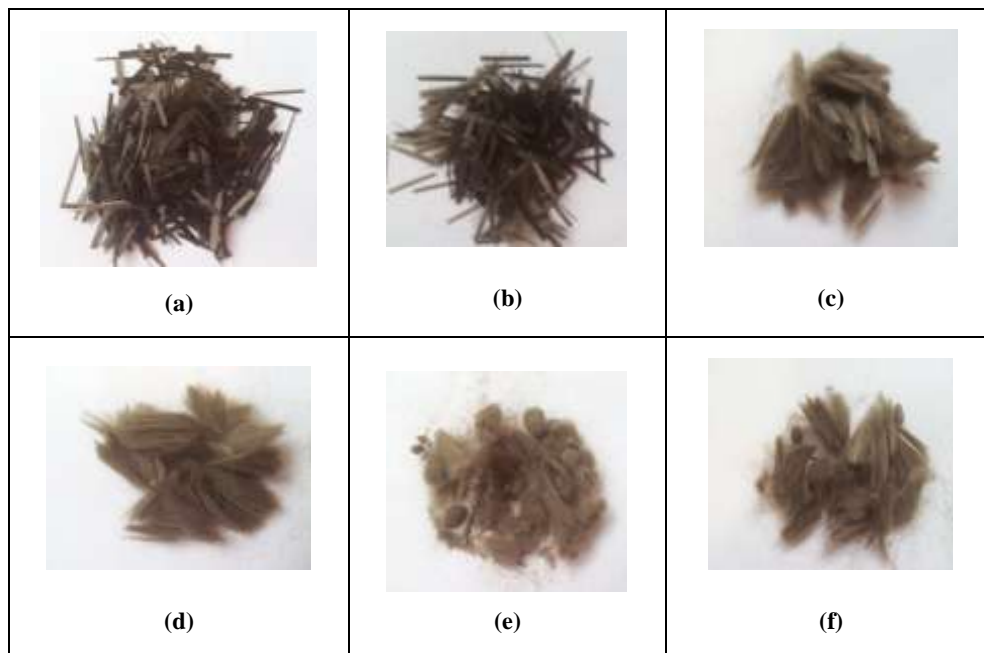
Figure 3. BF after 62 days of treatment with a) 3% NaCl (b) 10 % Na 2 SO 4 (c) 1 M NaOH (d) 1M NaOH + 3% NaCl (e) 1M NaOH +10% Na 2 SO 4 (f) 1 M NaOH+10% Na 2 SO 4 +3 %NaCl.
