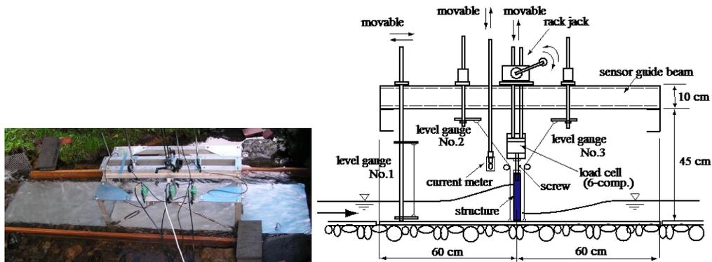
Figure 1. Experimental setup (left), and arrangement of structure and sensors (right).
