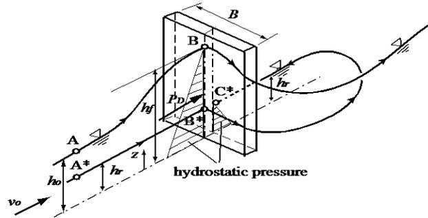
Figure 5. Assumed stream lines and hydrostatic pressures on the front and rear faces.
