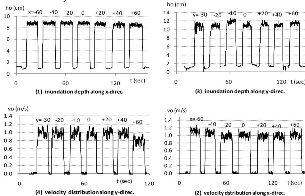
Figure 2. Distributions of inundation depth and velocity along and across the stream.
