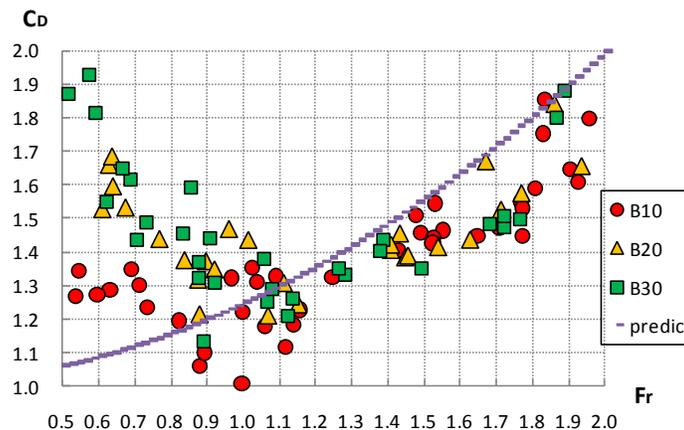
Figure 3. Drag coefficient of an isolated wall standing in non-overflow inundation.
