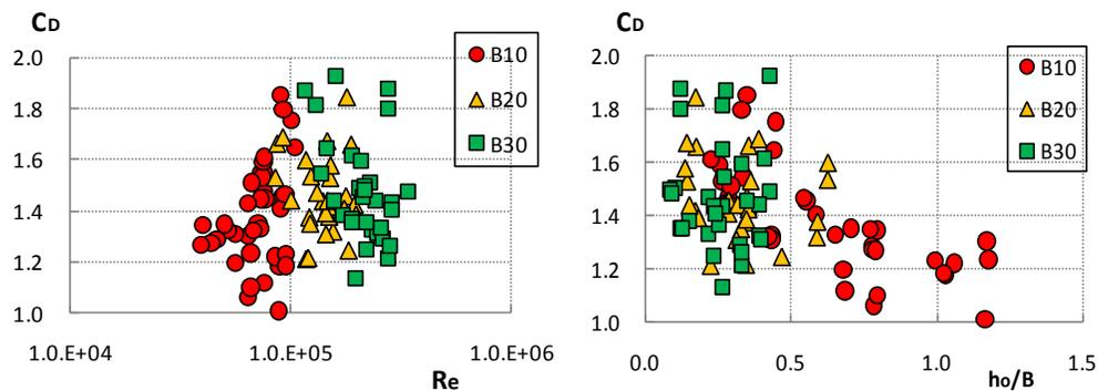
Figure 4. Effects of Reynolds number and aspect ratio on drag coefficient.
