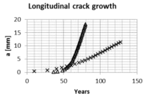
Figure 9. Longitudinal crack growth: A comparison with or without residual stresses.
