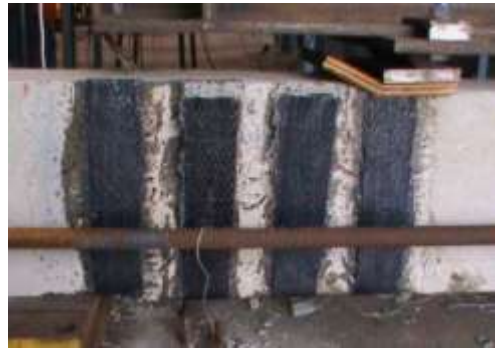
Figure 4. CFRP delamination and shear failure of beam specimen.
