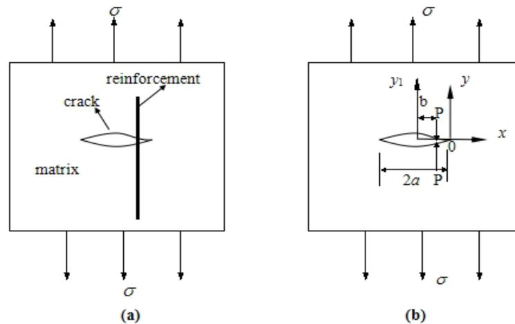
Figure 1. The problem and its mechanical model (a) $\Rightarrow$ (b).
