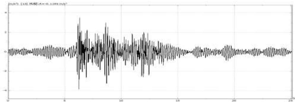
Figure 6. Acceleration response at the top floor in the  $y$ -direction.
