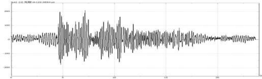
Figure 3. Strain response at the column foot in the  $x$ -axis.
