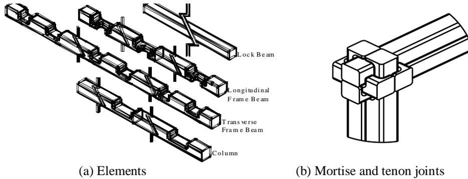
Figure 1. Assembly space frame and its components.
