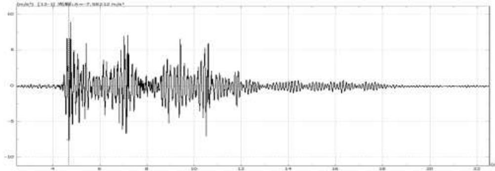
Figure 5. Acceleration response at the top floor in the  $x$ -direction.
