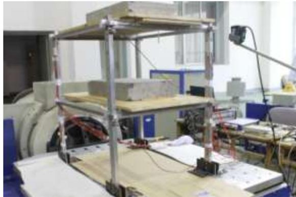
Figure 2. Frame model and shaking.
