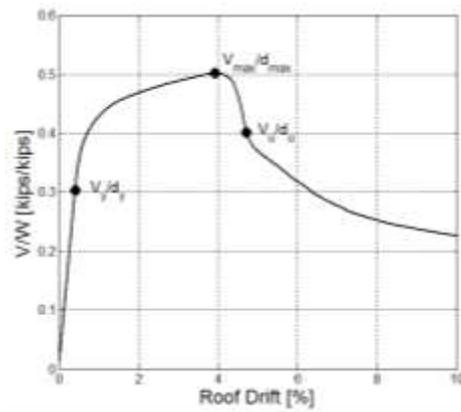
Figure 3. Nonlinear Static Analysis Pushover Curve of 8-story SPSW.
