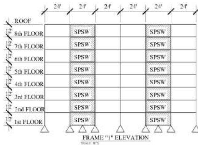
Figure 1. Elevation of the eight-story steel plate shear wall building.
