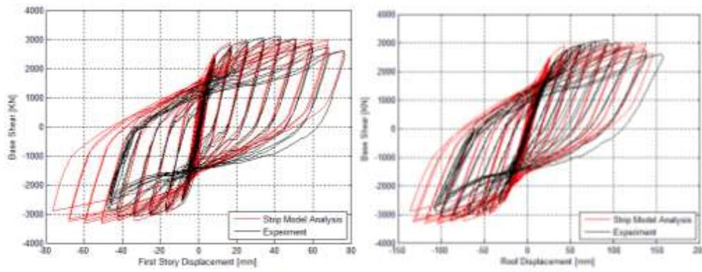
Figure 2. Hysteretic Material - Hysteresis Loop: (a) base shear vs. first story displacement; (b) base shear vs. roof displacement.
