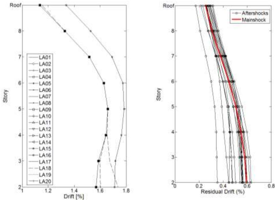
Figure 5. a) Inter-story Drifts for LA27+DBE; b) Residual Drift Results for LA27+DBE.
