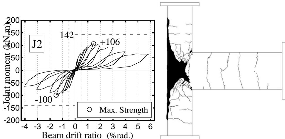
Figure 6. Joint moment–beam deflection relationships with final damage of J2.
