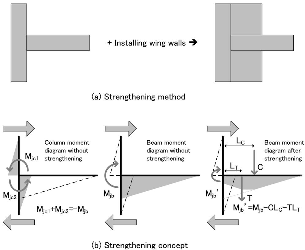
Figure 3. Concept to prevent joint failure by installing wing walls.
