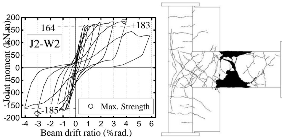
Figure 7. Joint moment–beam deflection relationships with final damage of J2-W2.
