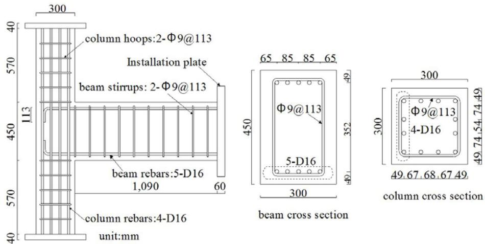
Figure 4. Dimensions and reinforcement details of the existing part of the specimens.
