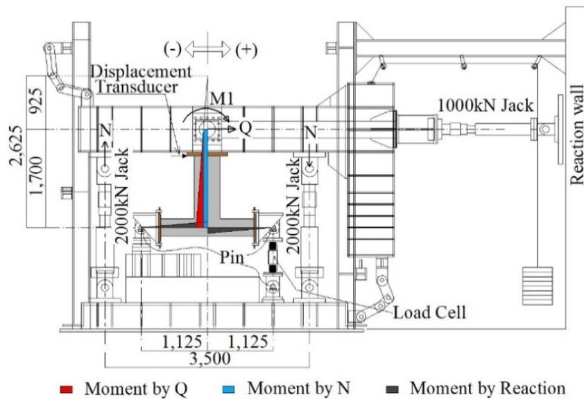
Figure 5. Schematic view of test set-up.
