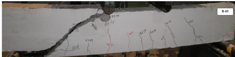
Figure 6. Failure mode of beam exposed to the tropical climate.
