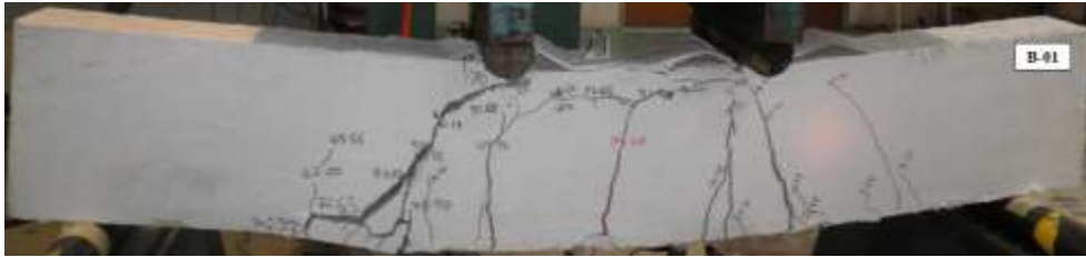
Figure 5. Failure mode of the control beam.
