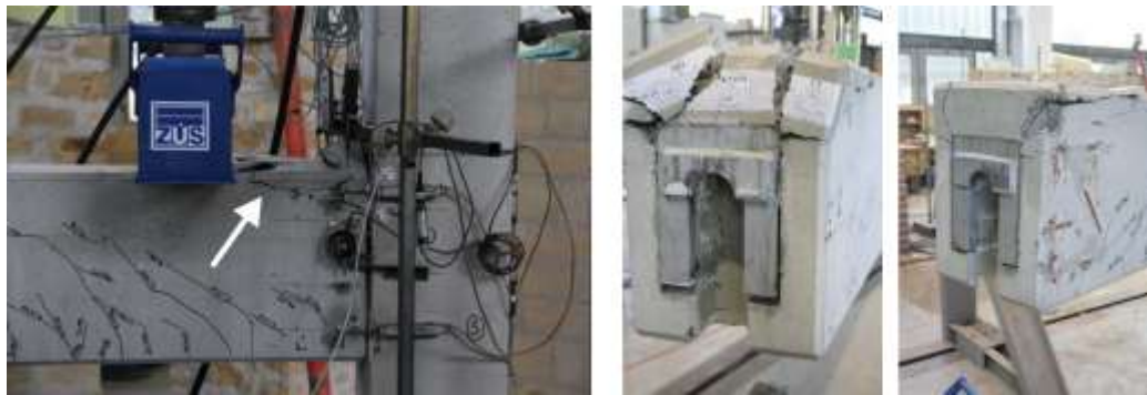
Figure 7. Failure of tested structure after static loading.
