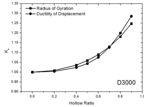
Figure 5. Ratio of ductility and radius of gyration (D3000).
