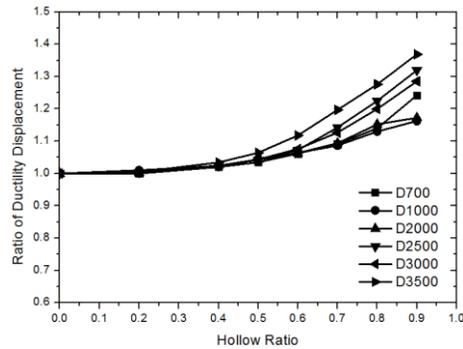
Figure 3. Ratio of ductility of displacement by diameter.
