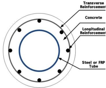
Figure 1. Section of composite hollow RC column.
