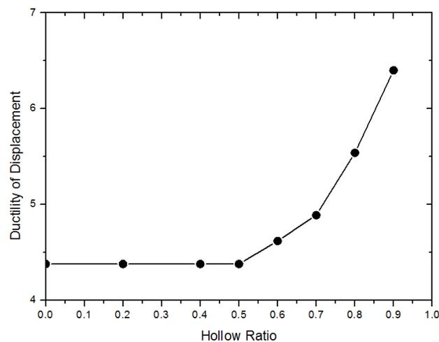
Figure 2. Ductility of displacement by hollow ratio.
