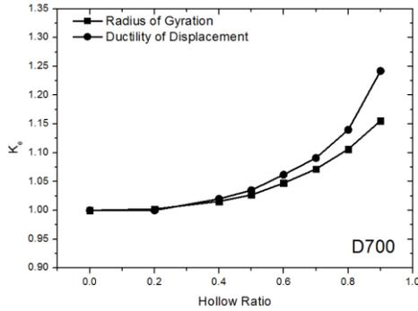
Figure 4. Ratio of ductility and radius of gyration (D700).
