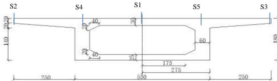
Figure 1. The cross-section dimensions of the skewed box-section girder bridge (Unit: cm).
