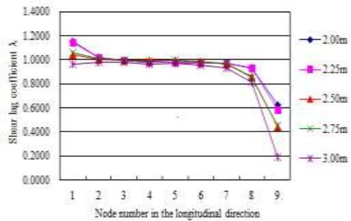
Figure 9. Shear-lag coefficient at S3 section.
