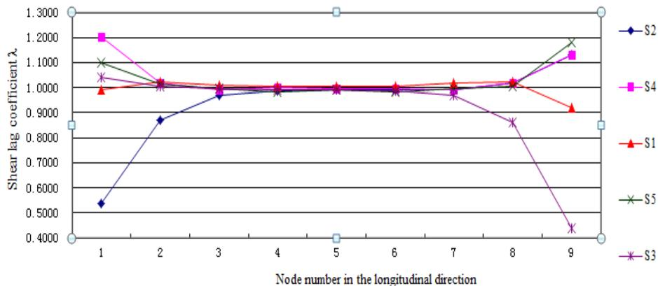
Figure 6. Shear-lag coefficients of five typical sections along the longitude.
