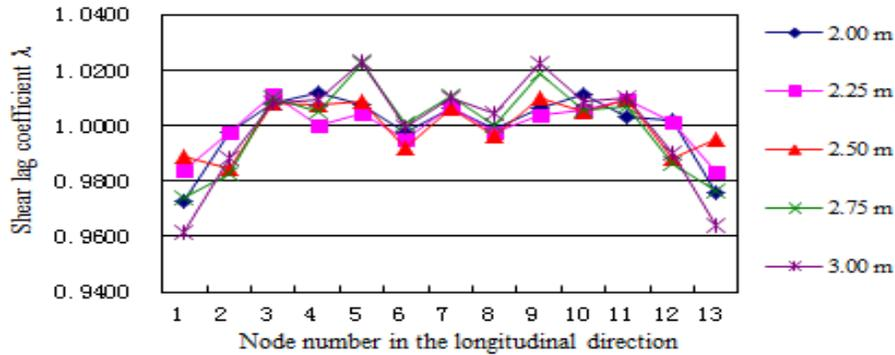
Figure 5. The shear-lag coefficients of the mid-span cross-section for different flange width.
