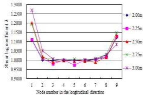
Figure 10. Shear-lag coefficient at S4 section.
