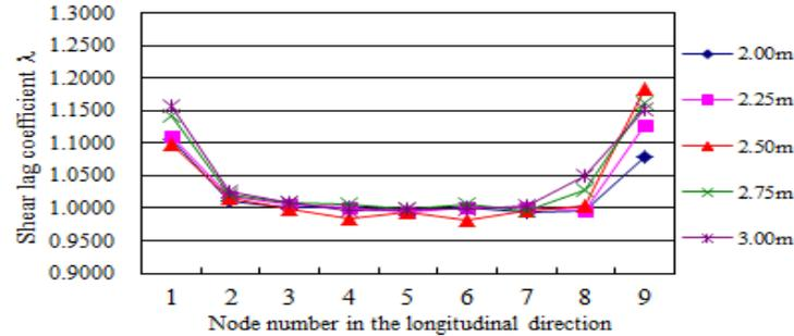
Figure 11. Shear-lag coefficient at S5 section.
