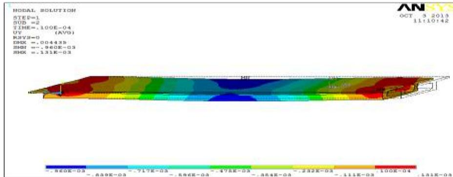
Figure 3. The bridge deformation for flange width of 2.00 m.
