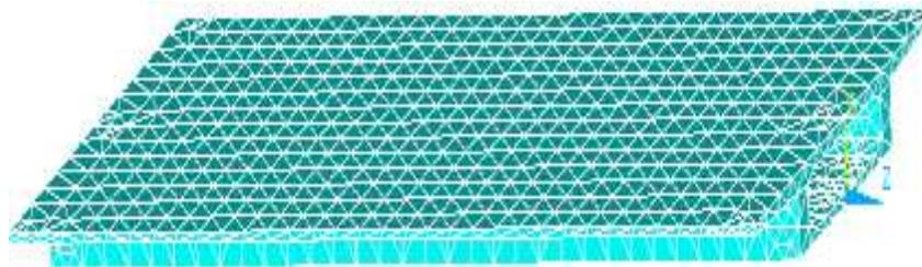
Figure 2. FE model of skewed box-section girder bridge.
