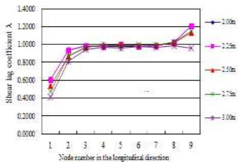
Figure 8. Shear-lag coefficient at S2 section.
