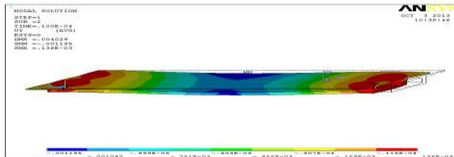
Figure 4. The bridge deformation for flange width of 3.00 m.
