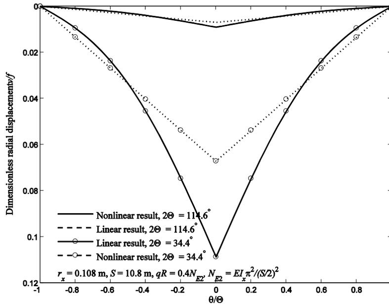
Figure 2. Comparison of distributions of radial displacements.
