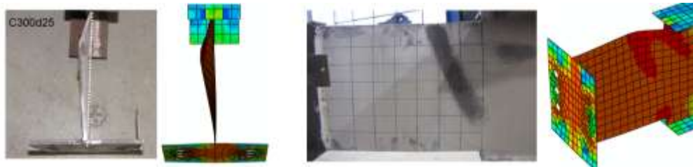
Figure 3. Typical buckling mode – test and FE results.
