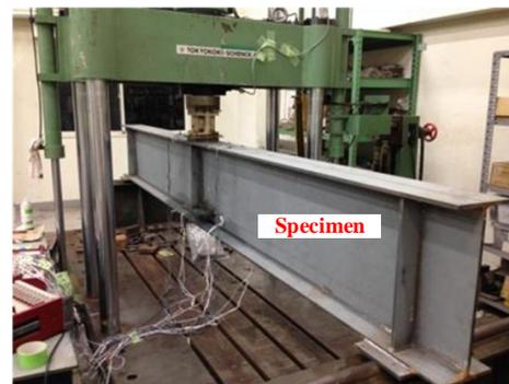
Photo 1. Loading test set up.
