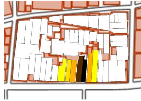
Figure 9. Fire spreading simulation result after 5 hours (Installation of fireproof wall in every third wooden house).
