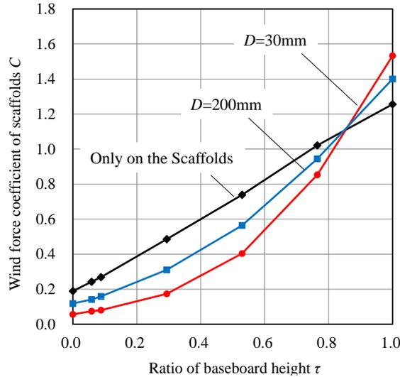
Figure 6. Relationship between the wind force coefficient and the ratio of the baseboard height.
