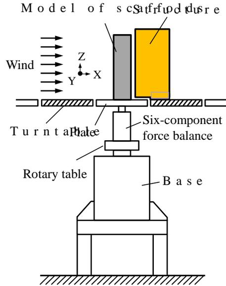
Figure 3. Six-component force balance.
