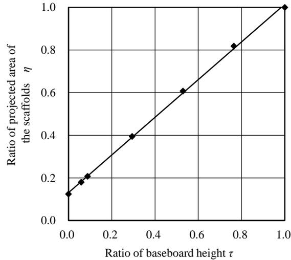
Figure 5. Relationship between the ratio of the projected area of the scaffolds and the ratio of the baseboard height.
