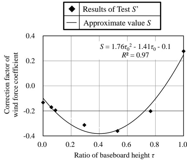
Figure 7. Relationship between the correction factor of the wind force coefficient of the scaffolds and the ratio of the baseboard height.
