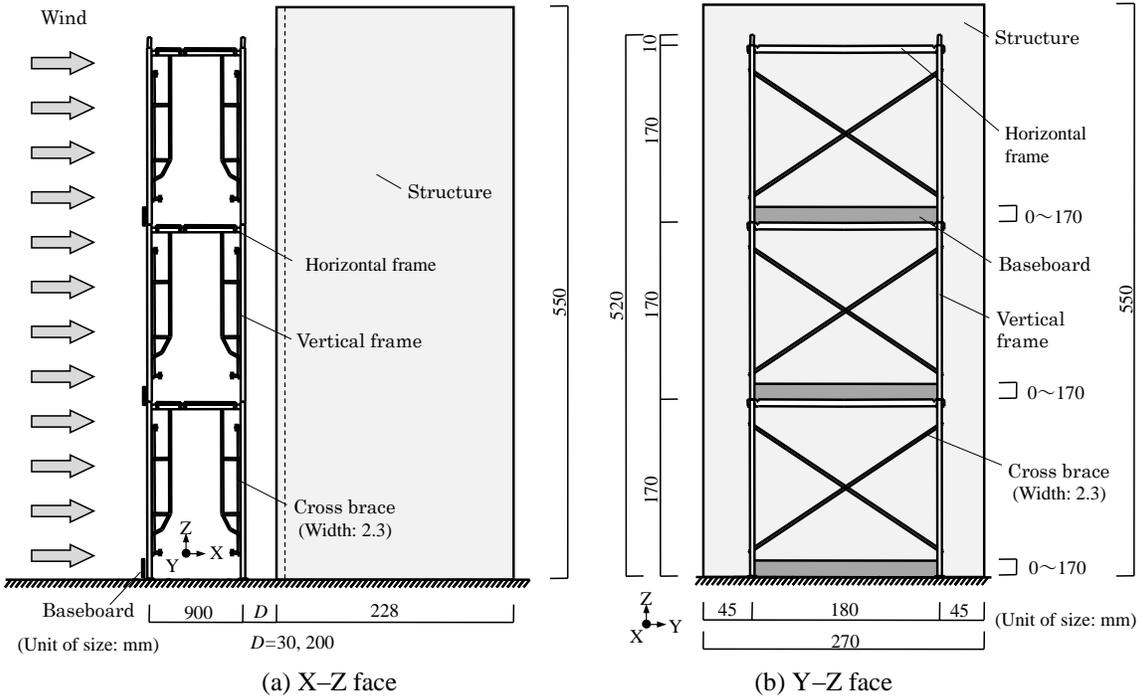
Figure 4. Scaffolds and structure used for the wind tunnel test.
