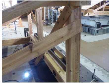
Figure 7. Buckling of brace (RA-4).
