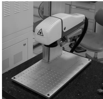
Figure 2. Appearance of the laser marking device.
