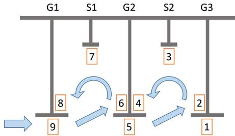
Figure 6. Installation position of dry gauze and the status of inflow wind.
