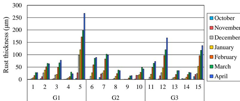
Figure 10. Rust thickness on exposed specimen.
