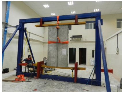
Figure 1. Light weight (LECA) concrete-filled cold formed steel wall specimen in the test frame.
