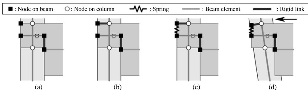
Figure 3. Example of modeling resistance for column-beam joint in positive loading.
