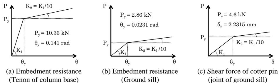
Figure 2. Examples of restoring force of resistance element.
