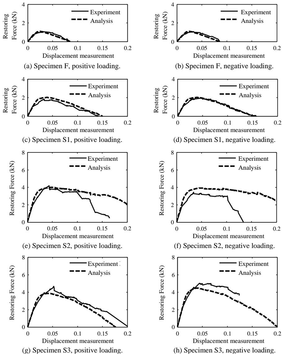
Figure 4. Simulation of skeleton curve on experimental result.
