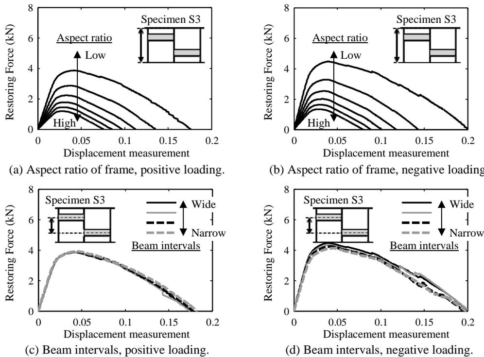
Figure 5. Sensitivity analysis of changing beam arrangement.
