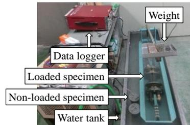
Figure 2. Test setup of the tensile creep test.
