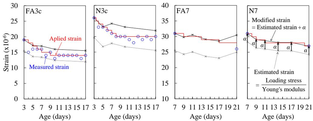
Figure 5. Decreasing elastic strains during the tensile creep test.
