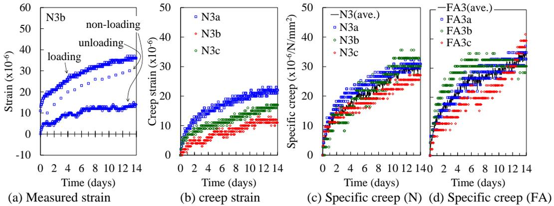
Figure 3. Strain behavior based on constant elastic strain.
