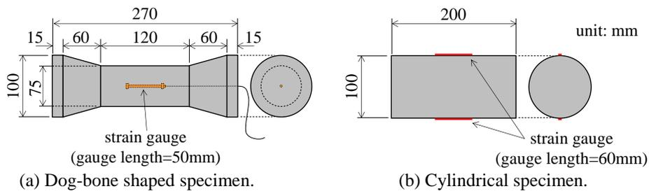
Figure 1. Dog-bone shaped specimen and cylindrical specimen.
