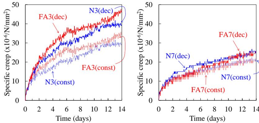
Figure 6. Specific creep based on the decreasing elastic strain.
