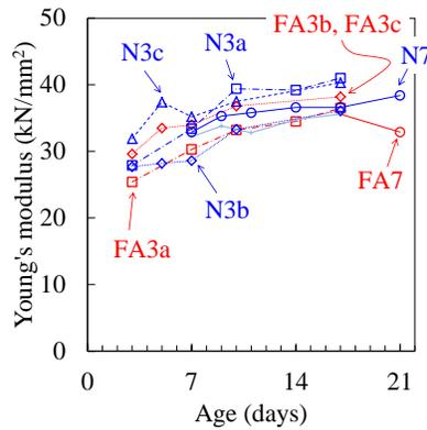
Figure 4. Young's modulus during the tensile creep test
