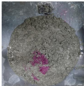
Figure 5. Slump flow 52cm of 45.5% of sand percentage.
