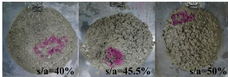
Figure 4. Result of T-post slump test.
