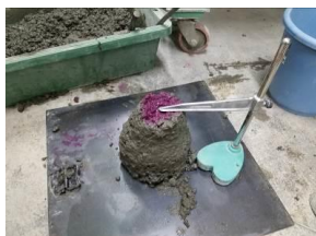
Figure 1. T-post slump test situation.
