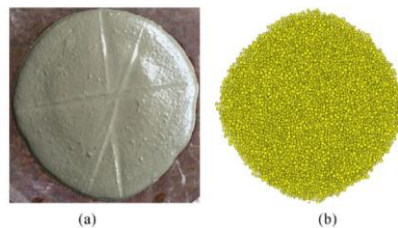
Figure 4. The final shape of the mortar on the flow table: (a) experiment (mean flow value: 210 mm), and (b) numerical simulation (mean flow value: 212mm) (Li et al. 2016).
