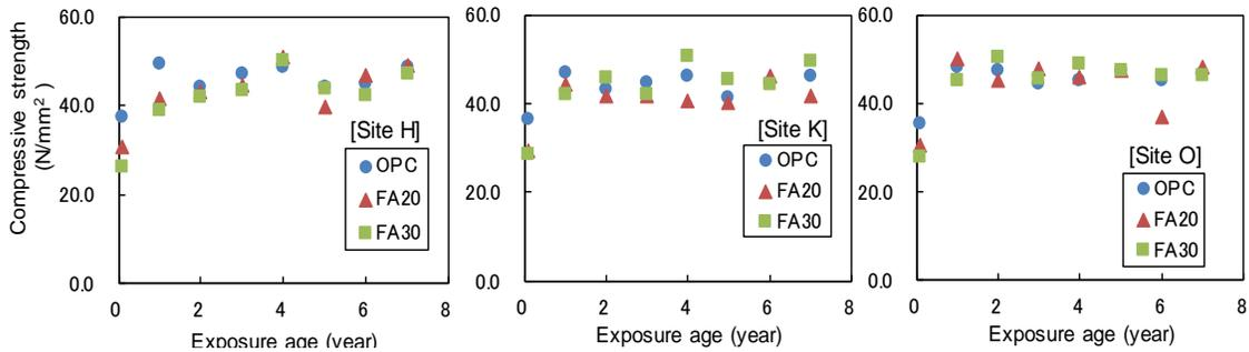
Figure 2. Changes in compressive strength with exposure age.
