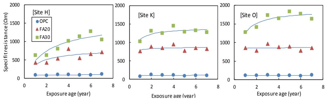
Figure 3. Changes in volume resistivity with exposure age.
