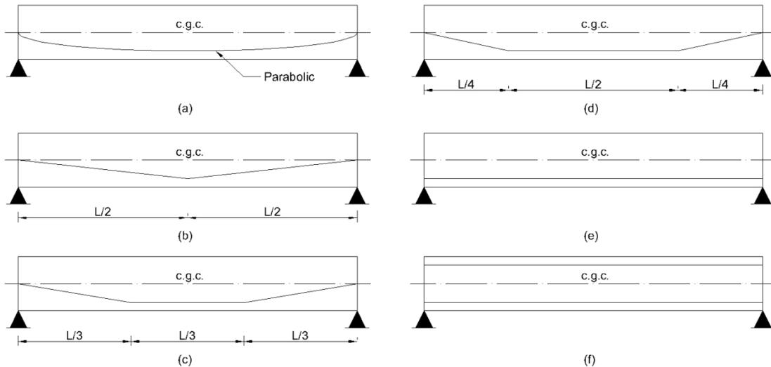
Figure 1. Profile of prestressed steel in flexural concrete members.
