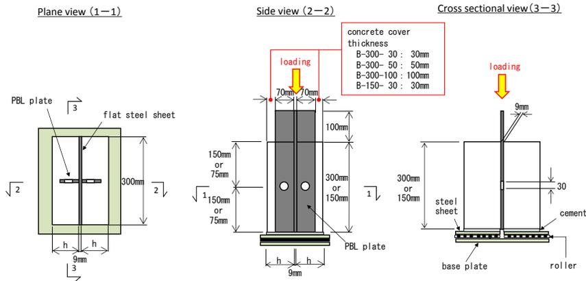
Figure 2. Specimen shape (B series).
