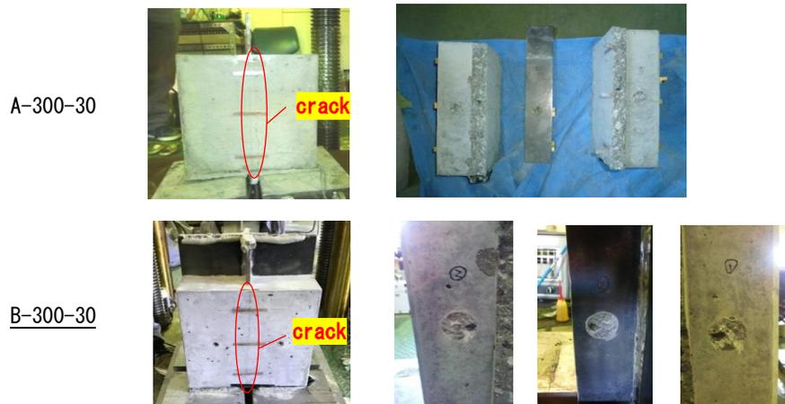
Figure 3. Specimen appearance after failure.
