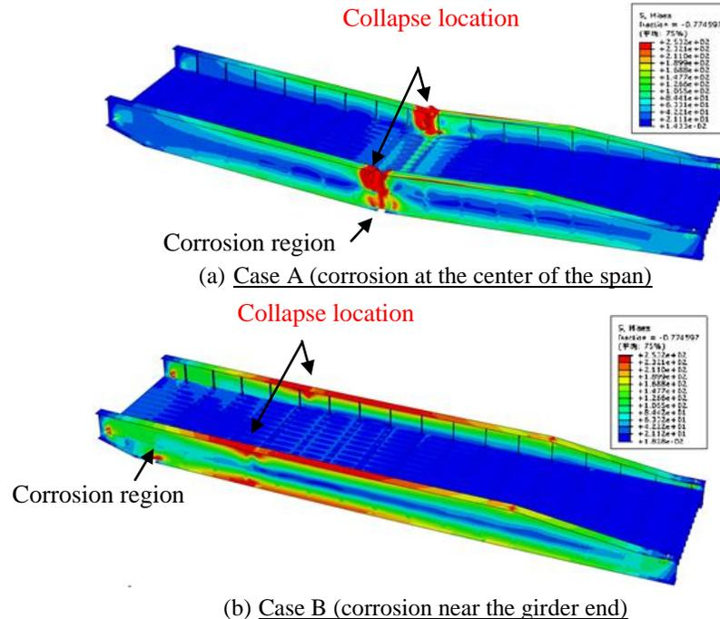
Figure 4. Collapse mode and von Mises stresses at maximum load.
