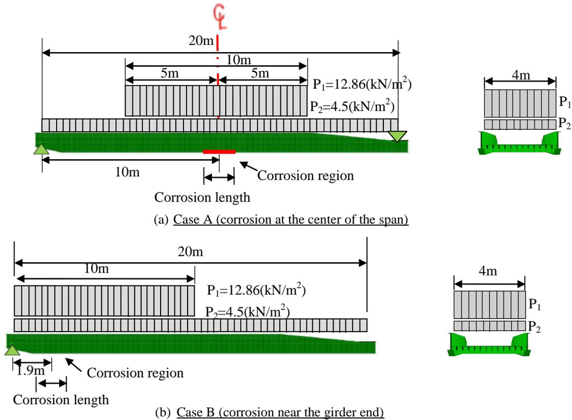
Figure 2. Location of live load (distributed L-load in JSBH).
