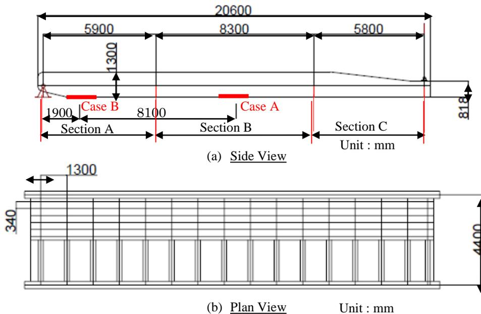
Figure 1. Dimensions of analyzed ferry bridge.
