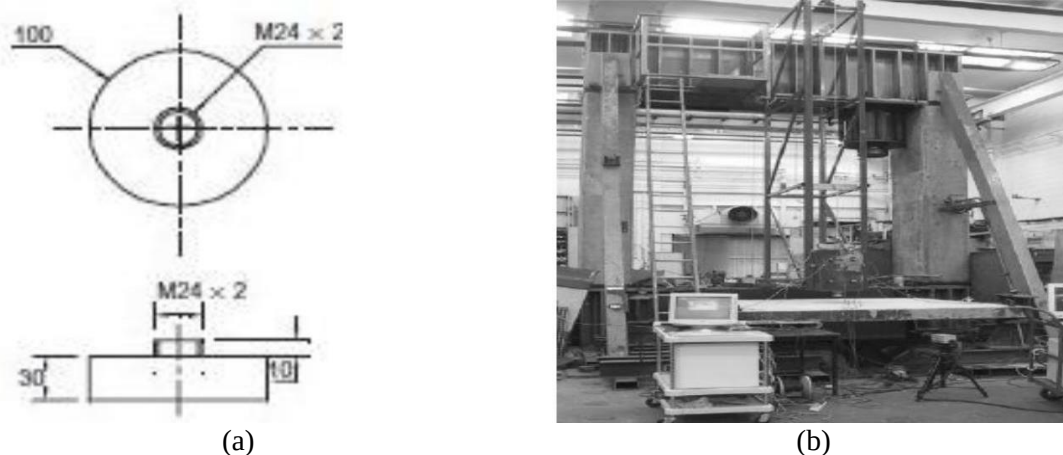
Figure 1. (a) Cross-sectional dimensions of impactor (b) impact test setup (Chen and May 2009).
