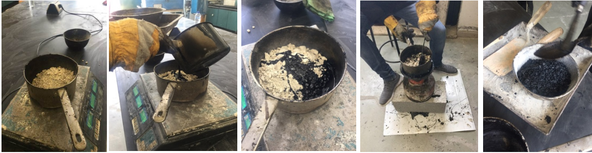
Figure 4. Mixing process of aggregates and bitumen with rubber.
