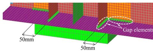
Figure 5. Modeling conditions of angle steels.
