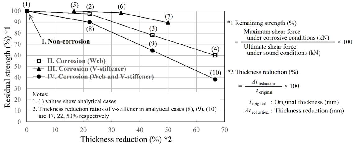
Figure 2. Shear capacity reduction due to thickness reduction.
