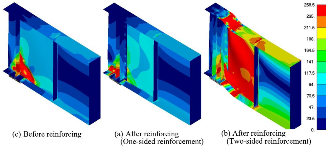
Figure 6. Von Mises stress distribution and deformed configurations at peak shearing force: Case (10).
