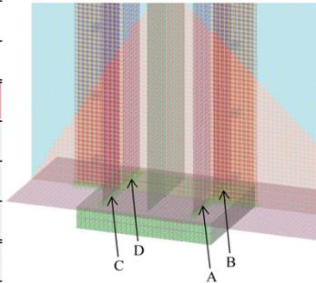
Note: The axial force that acts on an angle steel is calculated using the membrane stresses in the vertical direction on the elements at the lower end of the angle steel.
