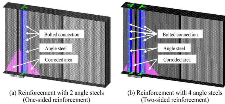
Figure 4. Analytical models after reinforcing.
