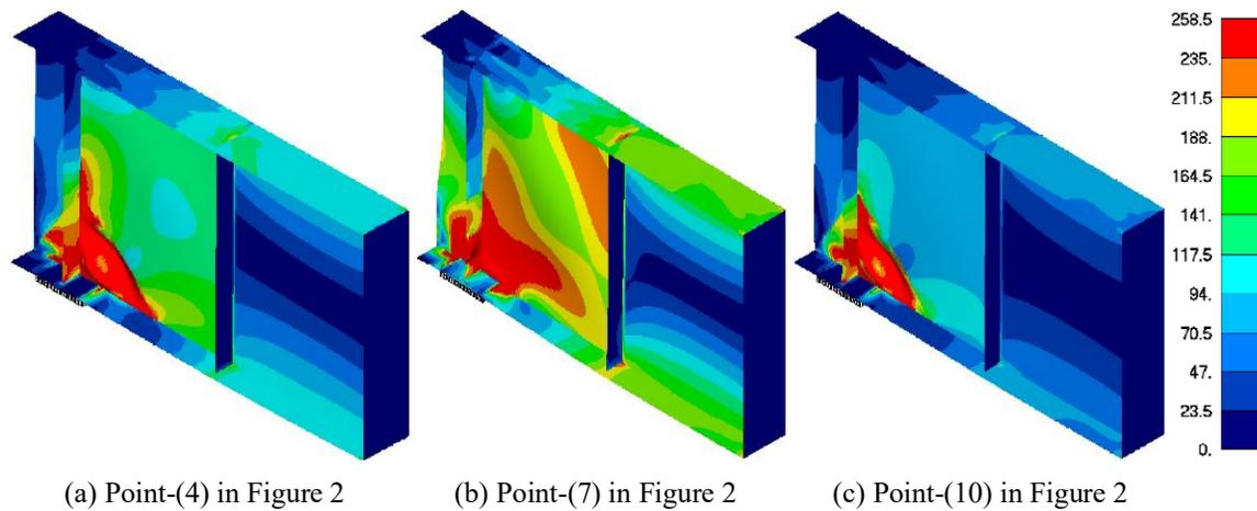
Figure 3. Von Mises stress distribution and deformed configurations at peak shear force.
