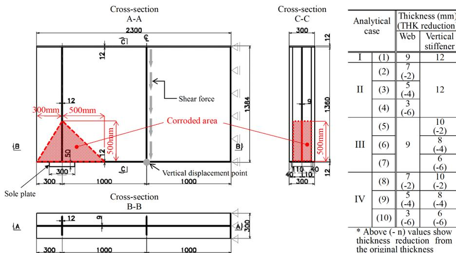
Figure 1. Girder dimensions used for analyses and the analytical cases (Incl. load and corrosion conditions).
