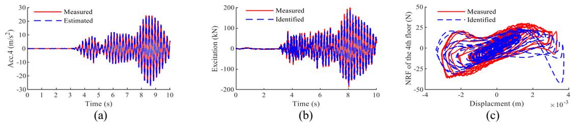
Figure 6. The comparison of identified results: (a) acceleration on the fourth floor, (b) excitation on the second floor, (c) the hysteretic of NRF on the fourth floor.
