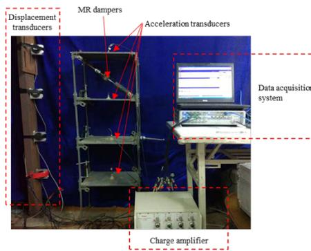
Figure 5. The experimental steel frame structure model.
