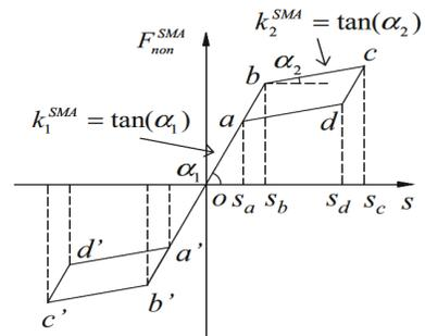
Figure 3. Hysteretic model of SMA damper.
