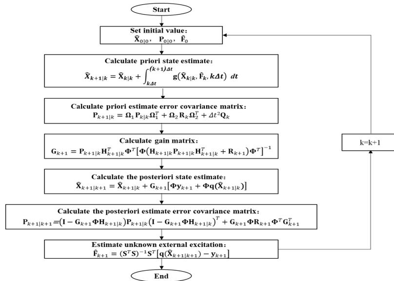
Figure 1. Identification flowchart of structural NRF and unknown excitations.
