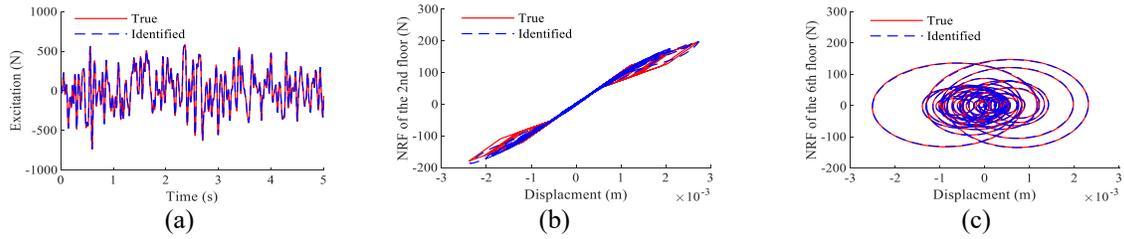
Figure 4. The comparison of identified results: (a) unknown external excitation, (b) the hysteretic of SMA damper on the second floor, (c) the hysteretic of MR damper on the sixth floor.
