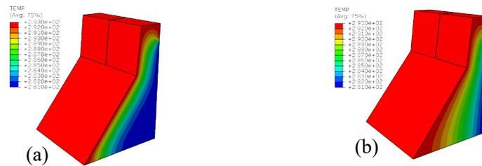
Figure 2. Variation of the temperature along the dam wall in Kelvin after a) 5 years and b) 20 years.
