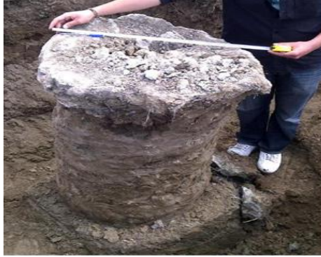
Figure 3. Trial column diameter measurement.
