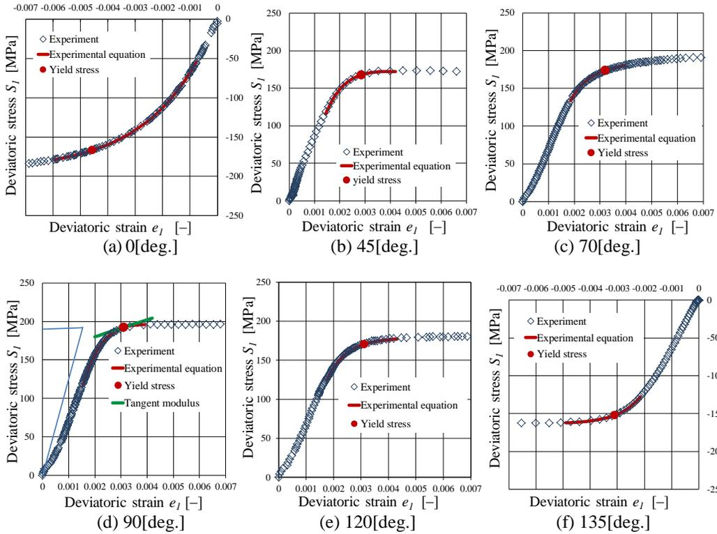
Figure 4. Principal deviatoric stress – deviatoric strain diagram.
