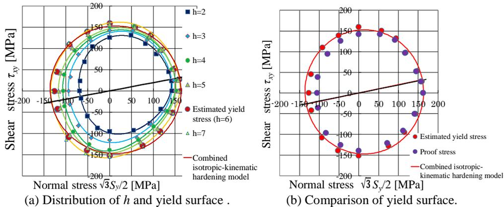
Figure 5. Shape of yield surface and distributions of strain hardening modulus  $h$ .
