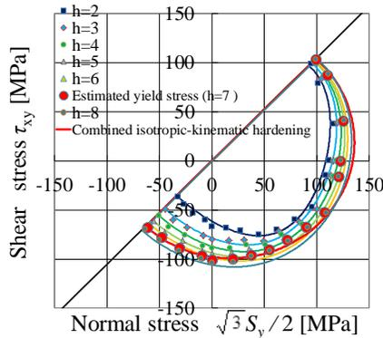
Figure 1. Distribution of  $h$  and yield surface in the case of proportional loading of tension and shear (the principal axis of pre-deformation;  $\theta = 65$  [deg.] and the final stretch is  $\lambda = 1.38$  [-]).
