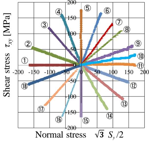
Figure 3. Stress points in each proportional loading tests.
