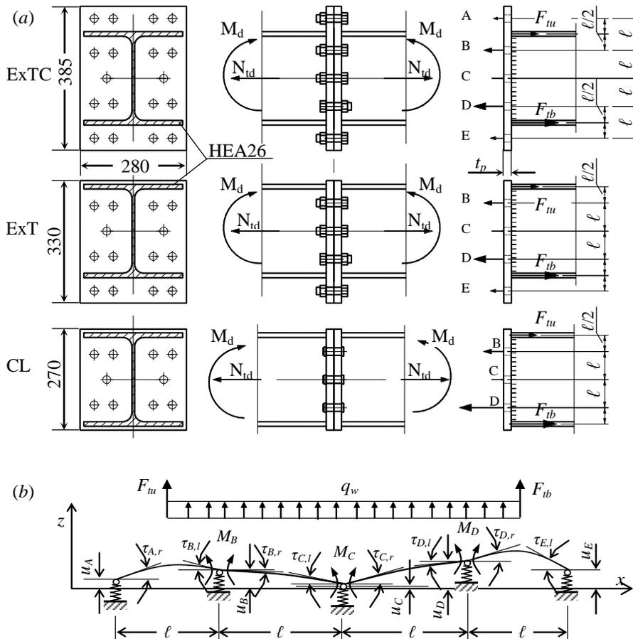
Figure 2. Tensioned splice joints: (a) structural variants ExTC, ExT, CL of splice joints ( $F_{tu}=401$  kN,  $F_{tb}=682$  kN,  $q_w=11.6$  kN/m); (b) design model of behavior of joint ExTC.
