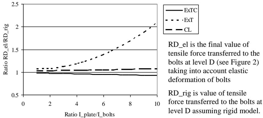
Figure 3. Relationship of force variation in bolts versus ratio of moments of inertia.
