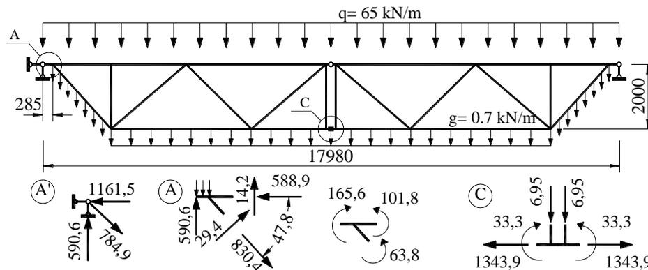
Figure 1. Rigid model of Warren truss and force diagrams for more attractive joints (axial forces in kN, bending moments in kNm).
