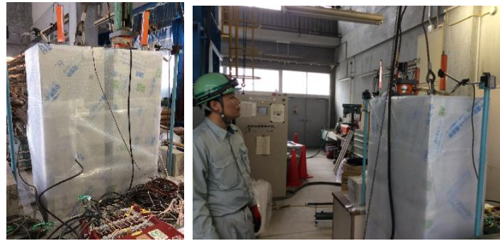
Figure 5. Test specimen covered with drying prevention and thermal insulating sheets.
